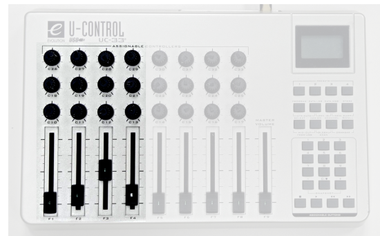
Figure 4: Relevant elements of the MIDI controller: The four leftmost columns control the parameters of the four synthesis processes.
